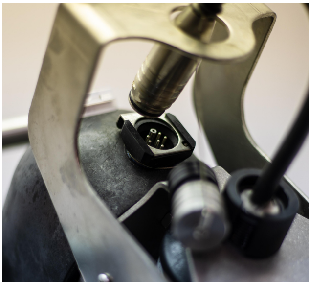
Figure 2-13 Secure caps and connect 310 ultrasonic plug to LaserFlow Ex
