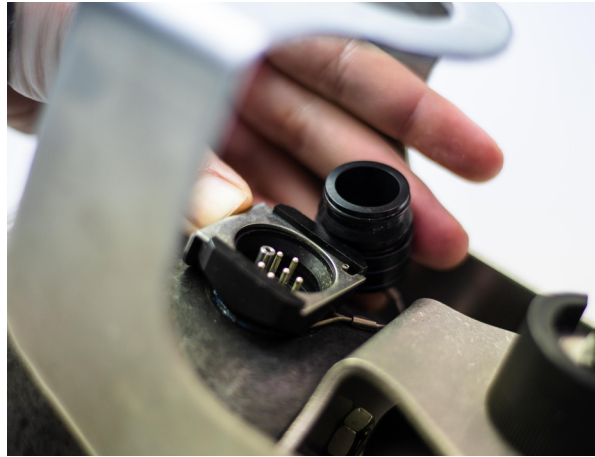
Figure 2-12 Preparing the LaserFlow Ex connector receptacle
